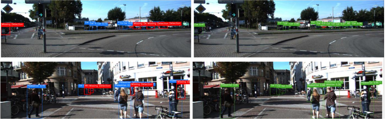
Fig. 3. Detection comparison on the KITTI test set: (a) baseline YOLOv12n and (b) YOLOv12n-SKNet
